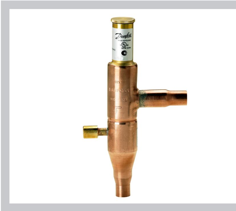
KVD is a modulating receiver pressure regulator. It opens on falling receiver pressure and bypasses hot gas to maintain the receiver pressure at the regulator setting (adjustable).
