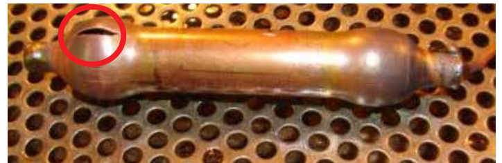
Burst areas observed 1 during the bursting pressure test
