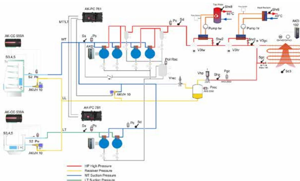
Figure 1: Example of mid-size supermarket installation with heat reclaim on the MT system.
