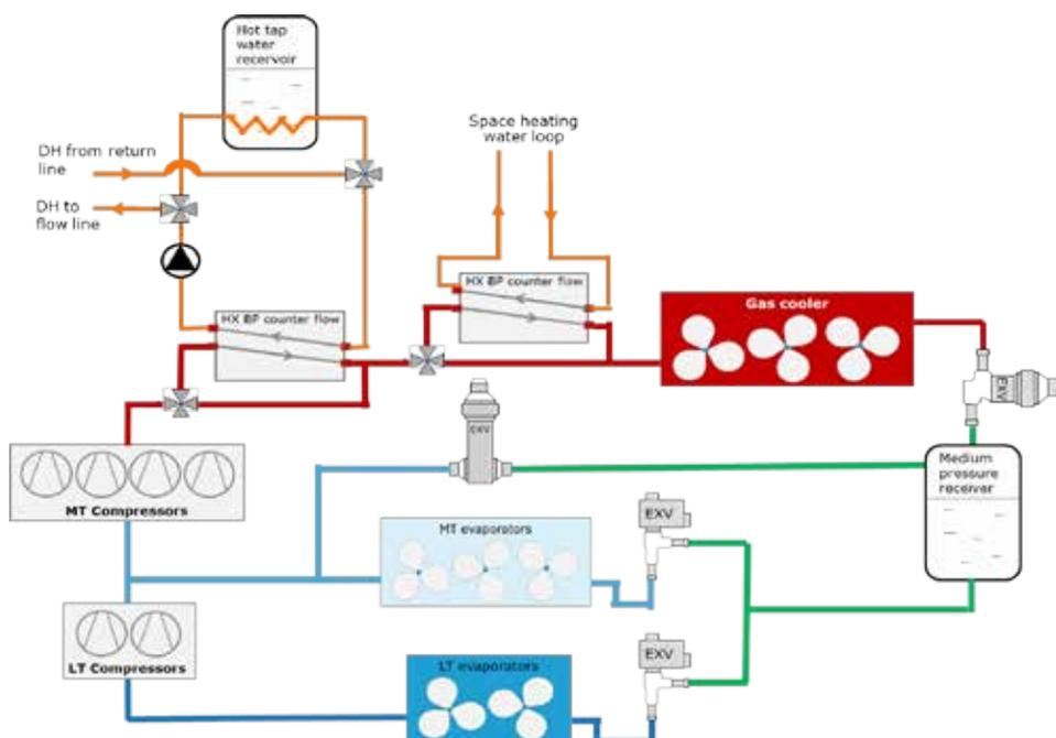
Figure 2: The concept of the CO<sub>2</sub> Transcritical system with heat reclaim and connection to district energy network
