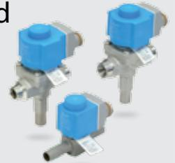
EVRS and EVRST stainless steel solenoid valves are based on three different principles: Direct, servo or forced servo operation. The forced servo operated valves, designed for keeping open at a pressure drop of 0 bar, can be used in liquid, suction, hot gas and oil return lines. EVRS and EVRST come equipped with a spindle for manual opening and have a working pressure of 50 bar and can handle media temperatures from -40 °C up to +105 °C (max temperature is dependent on coil).
