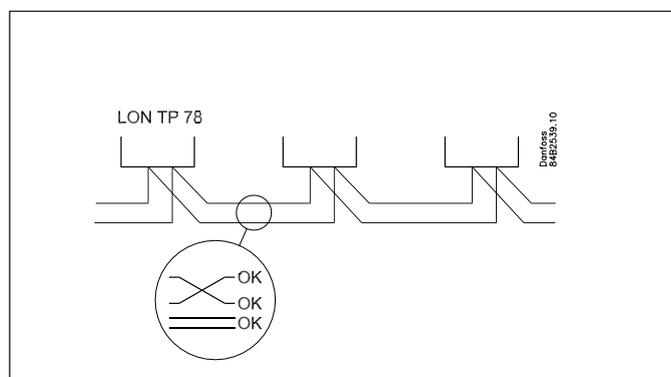
The two wires are looped from device to device. There are no polarisation requirements.
