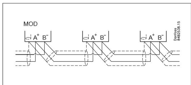
The wires are looped from device to device.
