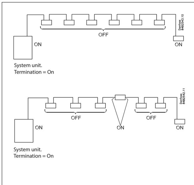
When all cables have been mounted on the different units, the cable must be terminated.
