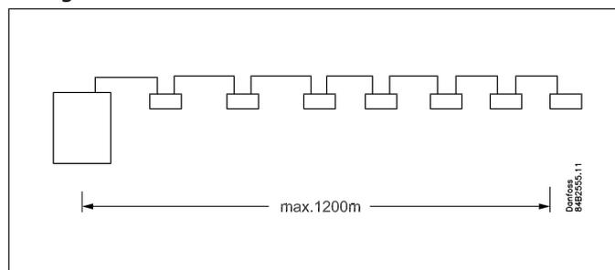
The cable is connected from controller to controller, and **no** branches are allowed on the cable.
