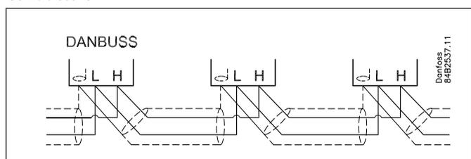
The wires are looped from device to device. L (K3) is connected to L (K3) and H (K4) to H (K4).
