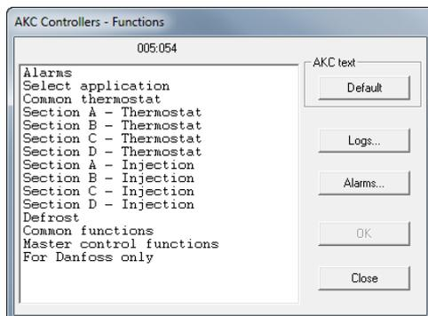
The operation is divided up into several function groups. When a selection has been made, push "OK", and you may continue to the next display. By way of example, "Common thermostat" has been selected here.
