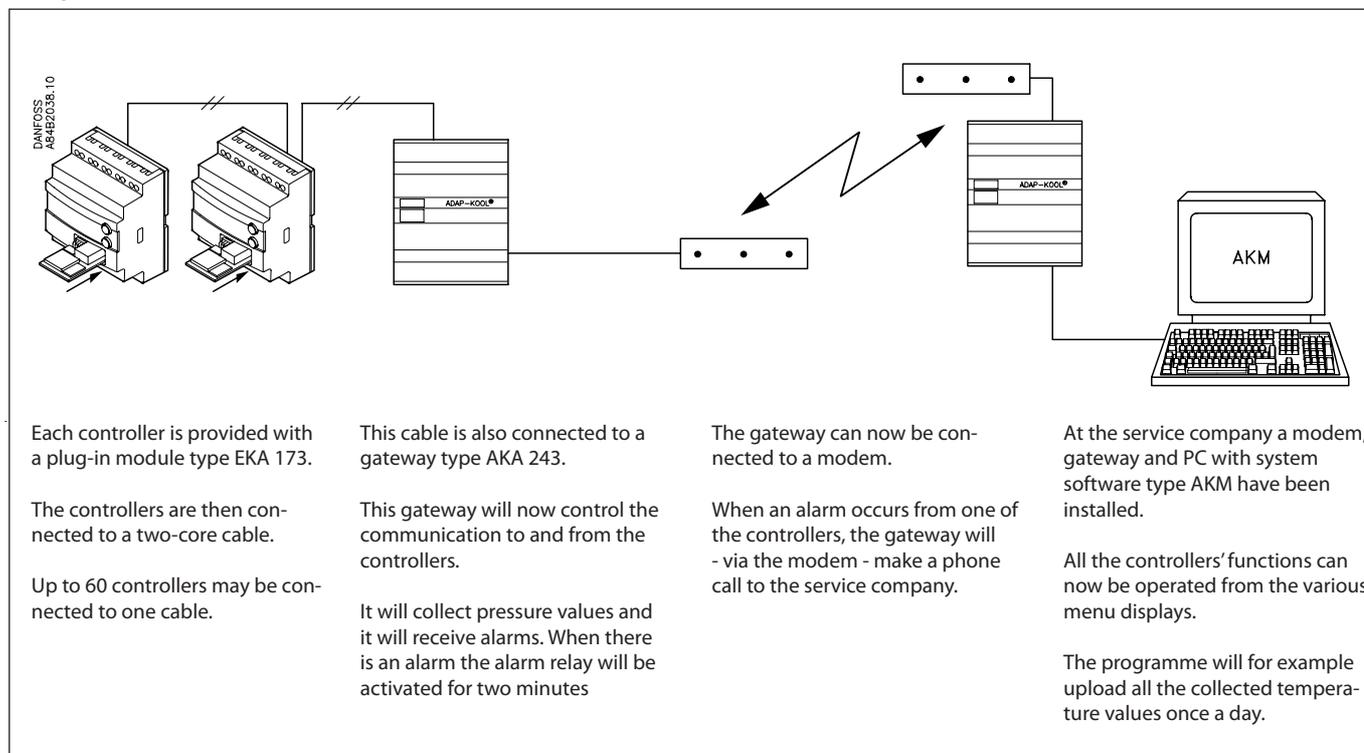
Each controller is provided with a plug-in module type EKA 173.
