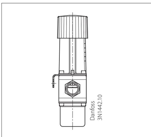
The valves can be installed in any position. An arrow on the valve body indicates the direction of flow. FJVA valves are also marked so that the letters RA can be read straightforwardly. The installation of an FV filter ahead of the valve is recommended.
