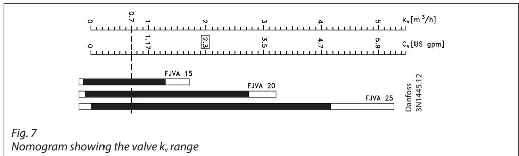
K<sub>v</sub> values are always given for water flow in [m<sup>3</sup>/h] with a pressure drop Δp of 1 bar.
