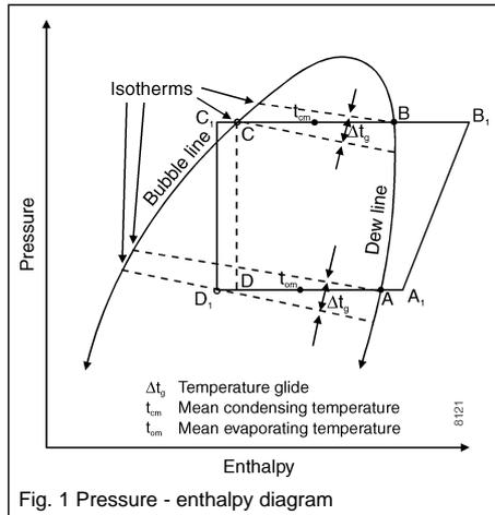
Fig. 1 Pressure - enthalpy diagram
