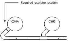
The 1-3/8" restrictor is used for SM115-125 units, the 1-5/8" restrictor is used for SM175-185. The restrictors are supplied with the compressors. The use of a restrictor is not necessary when
