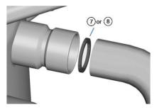
Place restrictor into suction connection, then braze suction line into place
