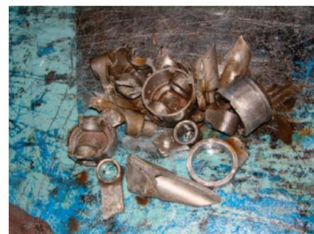
*Seized bearings, broken pistons and con rods even completely smashed compressors are all possible outcomes when the compressor is cycling on the Klixon because no overload protector has been fitted.*
