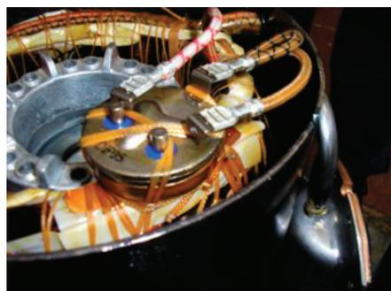
*Here we have a Klixon fitted to a 3-phase motor. The Klixon is the compressors last line of defence and should not be used to cycle the compressor.*
