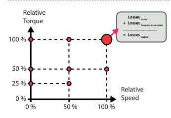
The system losses in the example are 1707 W, equating to efficiency class IES1.
