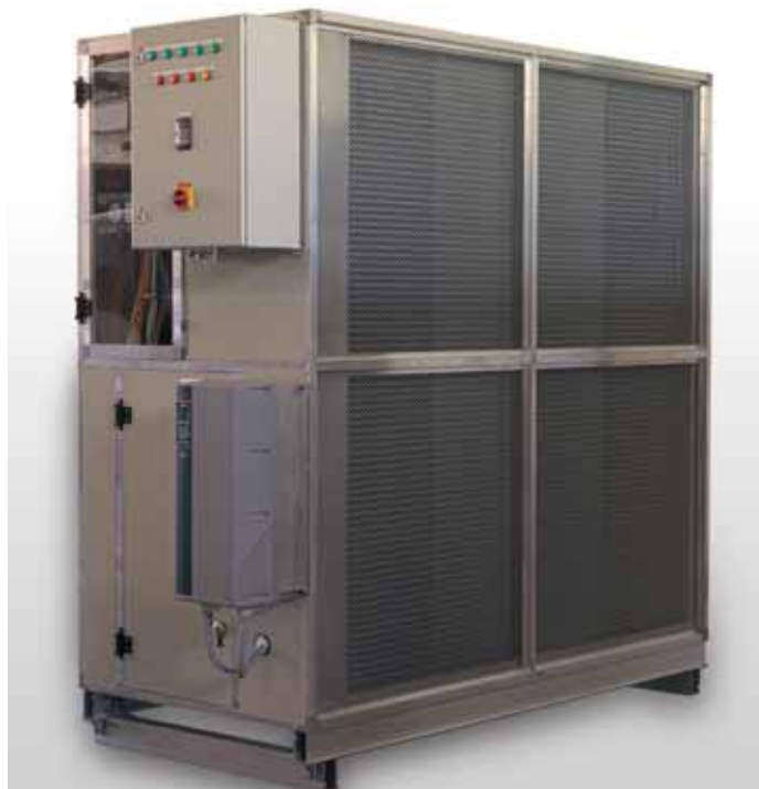
In the dehumidifier, the first heat exchanger extracts moisture by cooling air, and the water collects at the bottom. The second heat exchanger reheats the air and increases its capacity to absorb water vapor.
