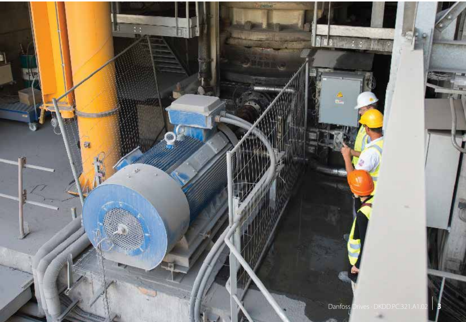
Direct coupling eccentric crusher driven by a 400-kW motor.
