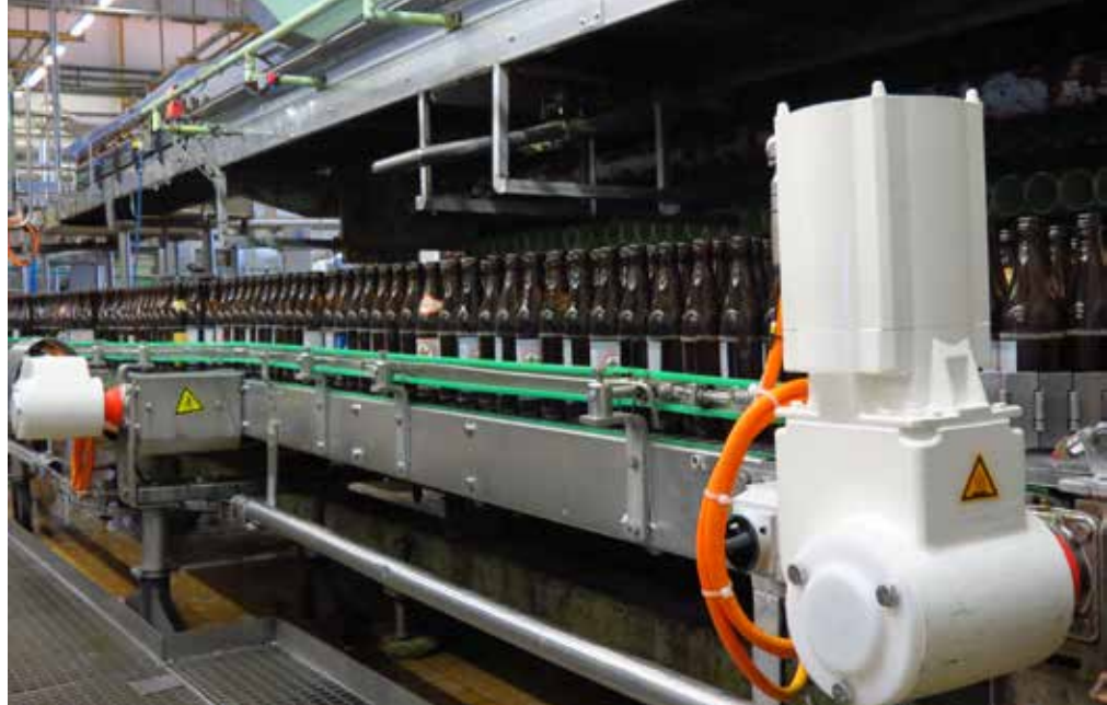
VLT® OneGearDrive® is mounted directly on the conveyor shaft.
