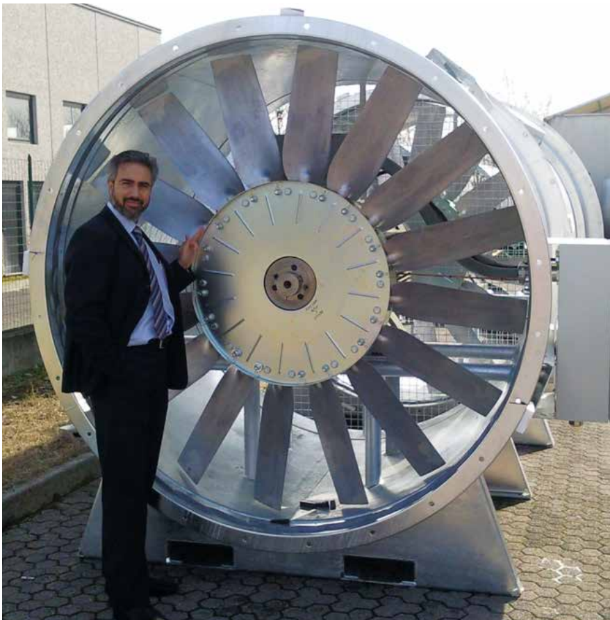
Roberto Redondi, Tunnel Construction Ventilation Manager at Systemair, with a 250 kW fan used for fresh air in the exploratory tunnel.
