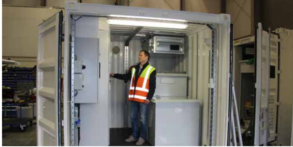
Sverre Knapstad with a new 450 kVA compact shore power supply fitted in a 10-foot container. The VACON® drives are adapted with controls and indicators required by the customer.
