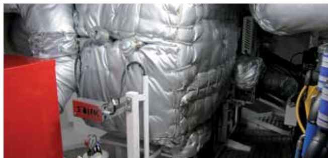
There are two 133 kW JohnDeere/Stamford generators in each engine room, four in total. The 2 engine rooms are located one at each end of the ship. The Solfic SCR exhaust gas filter removes toxic gases and particles.
