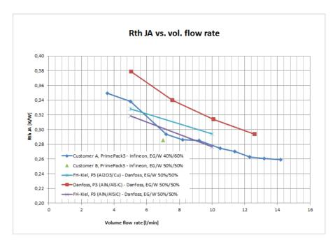
Thermal resistance, junction-water, for one single IGBT chip in the P3 module.
