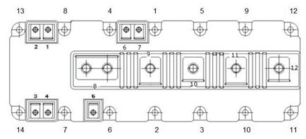
Recommended mounting sequence for the P3 module (Infineon/Danfoss).
