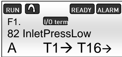
Figure 7.1-4, Low pressure alarm on the NXP panel
