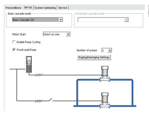
Illustration 11.6 View of Basic Cascade Control Set-up Tab
