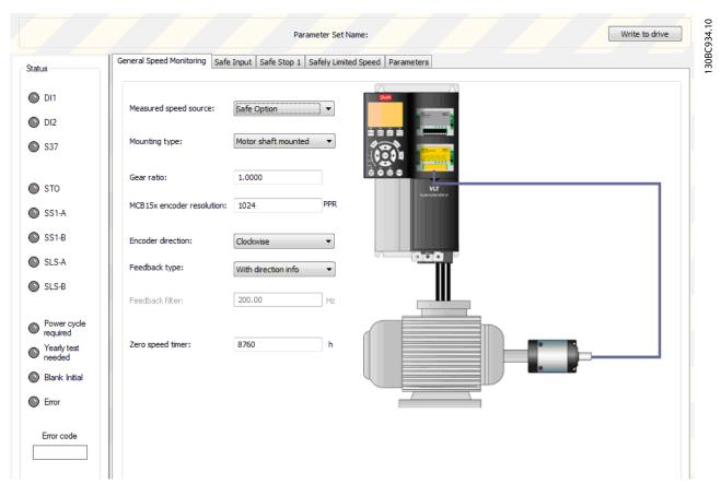
Illustration 13.3 The Opening Tab of the Safe Plug-in for VLT® Safety Option MCB 15x Series Plug-in Interface (Operating in Offline Mode)
