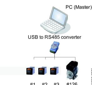
Illustration 1.1 Connect up to 126 nodes using a repeater. Without a repeater, connect up to 31 nodes.
