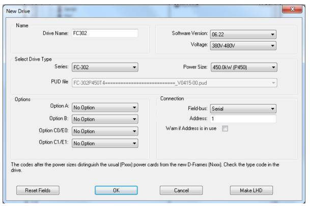
Illustration 5.5 Entering Data for a new Frequency Converter
