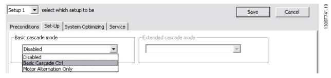
Illustration 11.5 Configuration Interface for Parameter Group 25-\*\* Cascade Controller
