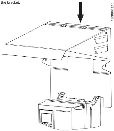
5. Fasten the shield to the bracket with two screws (max. tightening torque 5 Nm).
