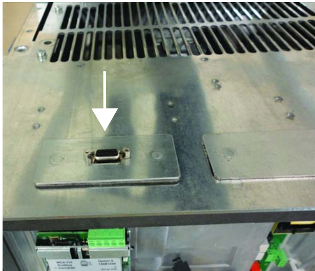
Illustration 1.5 Installing Sub D9 Cover Plate
