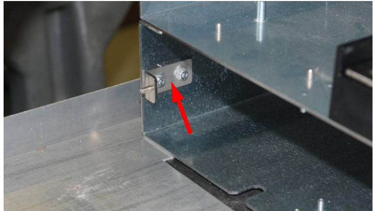
Figure 7. Mounting tab installed on left side of E2
