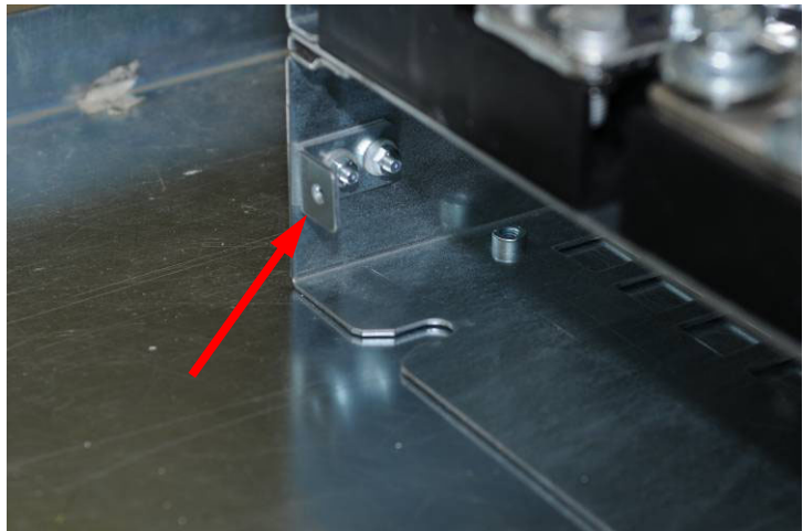
Figure 2. Mounting tab installed on left side of D3/D4 frame.
