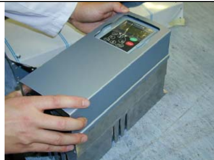
15. Fit the IP54 cover in its place. Keypad end first, then cable end.
