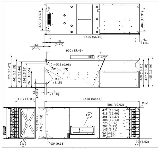
Fig. 6: Dimensions with the options module [mm (in)]
