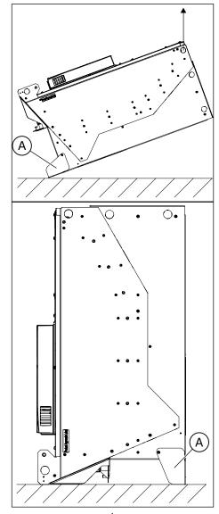
A. The support / fixing bracket
