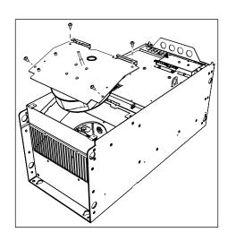
4 To release the fan from the cover plate, remove the 4 screws.
