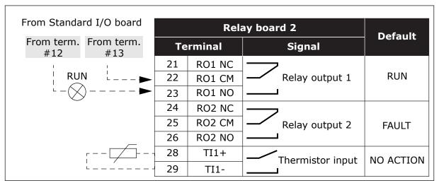
Fig. 28: The optional relay board (+SBF4)
