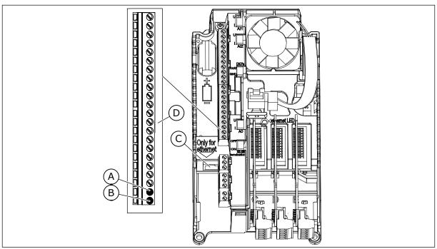
Fig. 31: The Ethernet and RS485 connections
