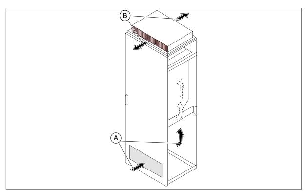
Fig. 22: The cooling air must move freely inside the cabinet
