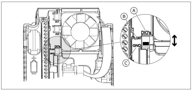
Fig. 30: Change the position of this switch to isolate the digital inputs from ground
