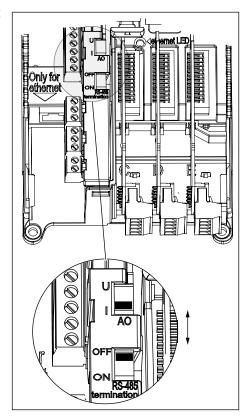
5 Set the bus termination for the first and the last device of the fieldbus line. We recommend that the first device on the fieldbus is the master device.
