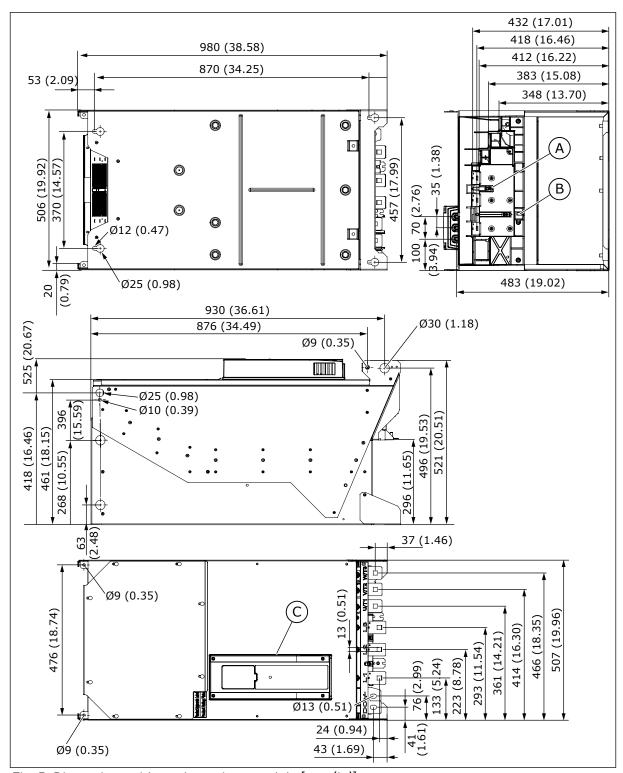
Fig. 5: Dimensions without the options module [mm (in)]
