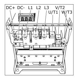
2 In MR12, connect the DC terminals of the 2 power units with the DC link cable. Connect the DC+ terminals together, and the DC- terminals together.
