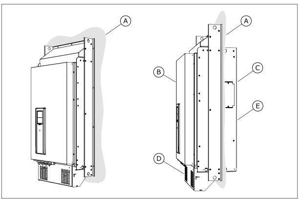
Fig. 18: Example of flange mounting (enclosure size MR9)
