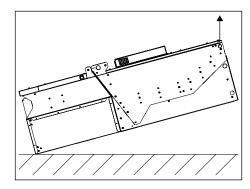
5 The maximum lifting angle is 60 degrees.
