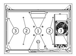
4 To release the fan from the cover plate, remove the 4 screws.
