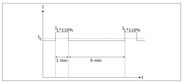
Fig. 37: Low overload in VACON® 100 FLOW
