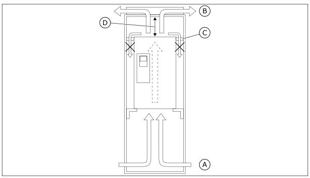
Fig. 21: The correct circulation of cooling air inside the cabinet
