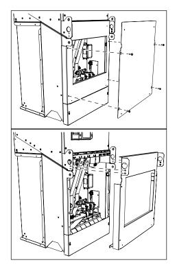
2 Find the EMC jumper between the terminals L2 and L3.
