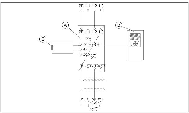
Fig. 12: The main circuit diagram, MR8 and MR9
