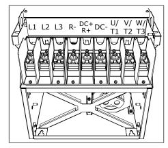
3 In MR12, connect the DC terminals of the 2 power units with the DC link cable. Connect the DC+ terminals together, and the DC- terminals together.
