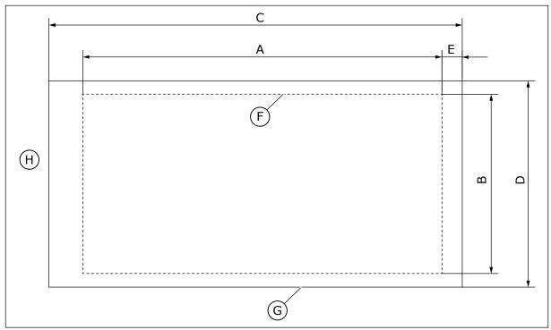
Fig. 19: The dimensions of the opening and drive module outline with flange
