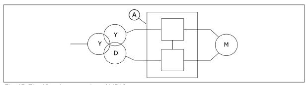
Fig. 17: The 12-pulse operation of MR12
