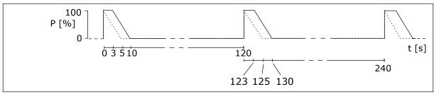
Fig. 36: The duty cycles of the LD and HD pulses
