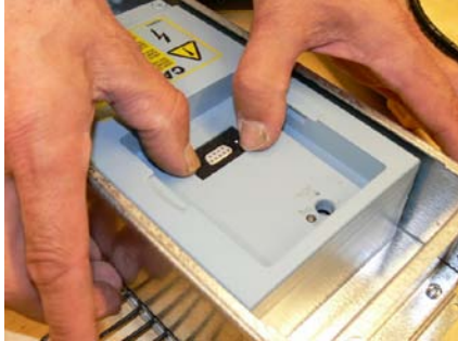
13. Attach the seal around the RS485 connector.
