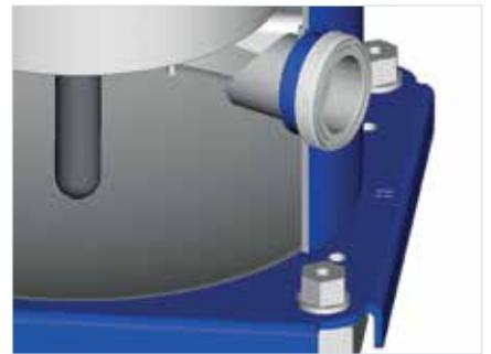
**The organ pipe** significantly improves system reliability by retaining oil in non-operating compressors under part-load operation in manifold configurations. Additionally, oil retention in the compressor improves the heat transfer in the evaporator, boosting overall system efficiency.
