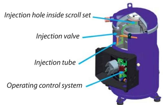
Fig. 1: Danfoss R32 compressor with liquid injection
