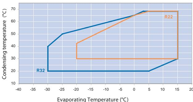
Fig. 3: Operating envelopes: comparison between R32 with liquid injection and R22 compressors
