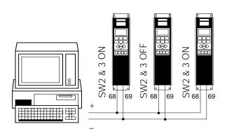
In order to avoid potential equalizing currents in the shield, the cable shield can be grounded via terminal 61, which is connected to the frame via an RC-link.
