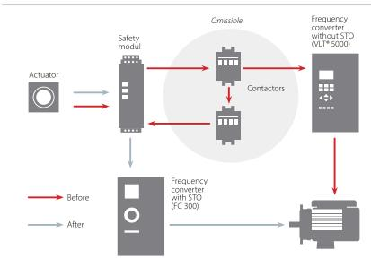
Two contactors can be omitted in safety installations due to the safety functionality in  $VLT^{\circ}$  Refrigeration Drive.
