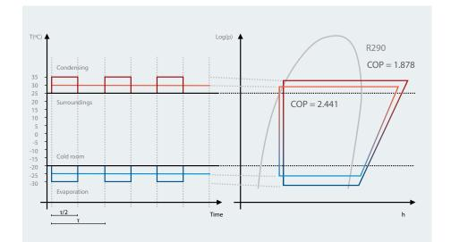
The figure on the left shows the condensation temperature curve (red) and the evaporation temperature curve (blue). The effect of on/off operational behaviour compared to a stable temperature (straight line) is
