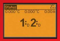
Read the compressor status directly from the display. D = Variable speed control, O = Off, F = Mains operation, X = Deactivated
