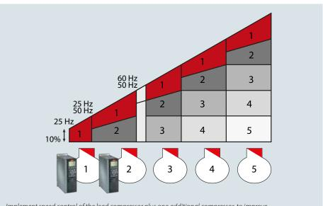
Implement speed control of the lead compressor plus one additional compressor, to improve and streamline design alternatives. The broader choice of compressor sizing enables adaptation to varying load conditions
