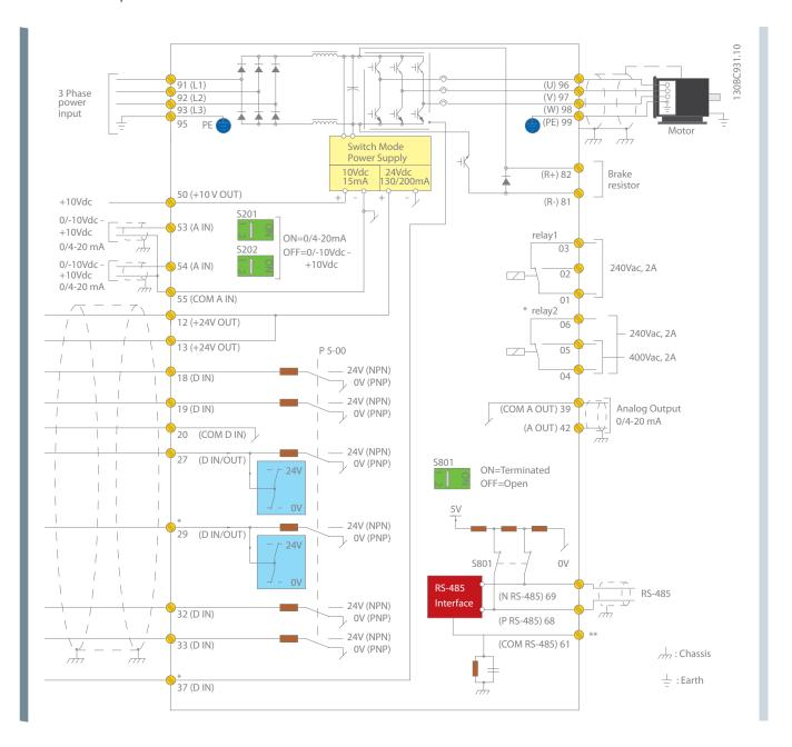
This diagram shows a typical installation of the VLT® Refrigeration Drive. Power is connected to the terminals 91 (L1), 92 (L2) and 93 (L3) and the motor is connected to 96 (U), 97 (V) and 98 (W).
