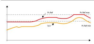
Floating condensing temperature set point control by VLT® Refrigeration Drive FC 103.
