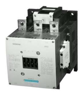
CONTACTOR, 250KW/400V/AC-3 AC(40...60HZ)/DC OPERATION UC 220-240V AUXILIARY CONTACTS 2NO+2NC 3-POLE, SIZE S12 BAR CONNECTIONS CONVENT. OPERATING MECHANISM SCREW TERMINAL
