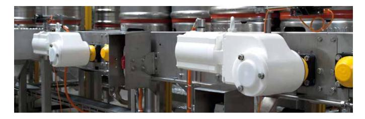
In line with the IE classification system for electric motors, the European standard IEC 61800-9-2 has been developed over the past few years. It defines IE efficiency classes for drives and IES classes for drive-motor systems.
