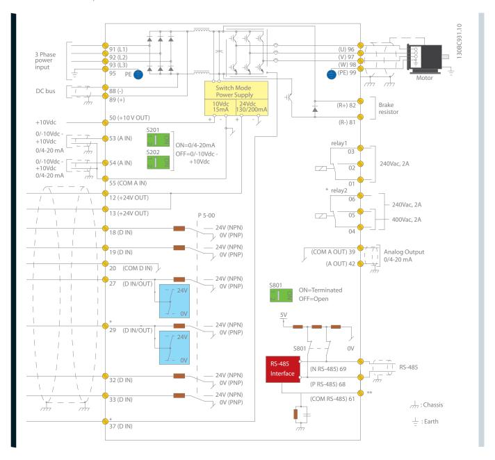
This diagram shows a typical installation of the VLT® AQUA Drive. Power is connected to the terminals 91 (L1), 92 (L2) and 93 (L3) and the motor is connected to 96 (U), 97 (V) and 98 (W).
