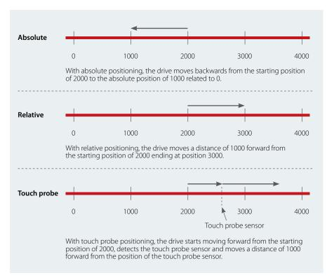
Fig. 3. IMC supports 3 positioning modes
