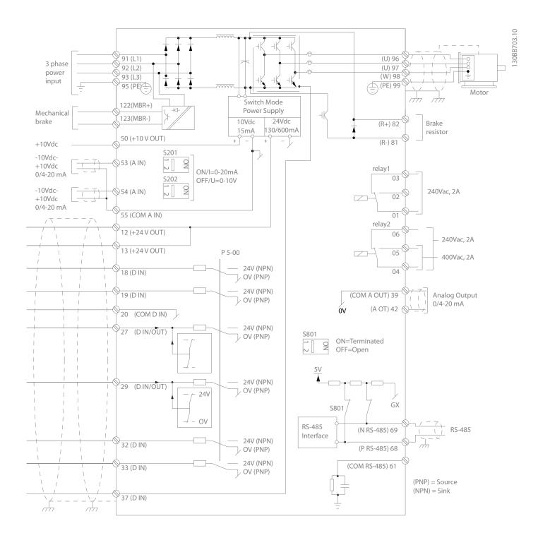
The diagram shows the port terminals of the FCD 302. Additional options will expand the number of terminals. The numbers indicated refer to the terminal numbers of the drives. Users can set the mode of the analogue inputs 53 and 54 by using the S201 and S202 switches.
