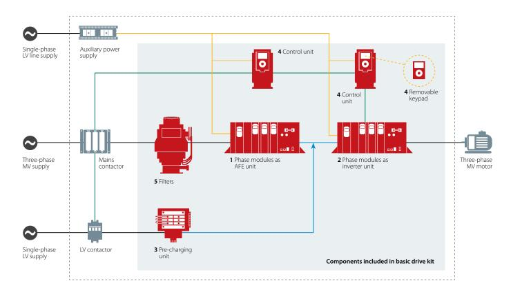
Example of VACON® 3000 Drive Kit: single line diagram for an AFE configuration.
