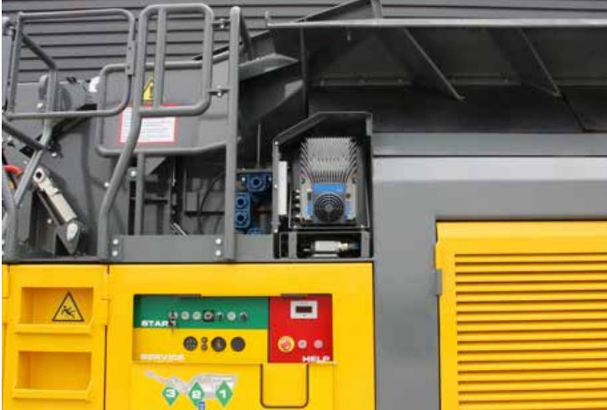
RUBBLE MASTER uses VACON® 100 X drives in their new mobile crusher RM V550GO! to control two unbalanced motors in parallel which run a vibrating conveyor. For RM, the VACON® 100 X provides a customized solution in a standard device, fulfilling all RM's requirements.
