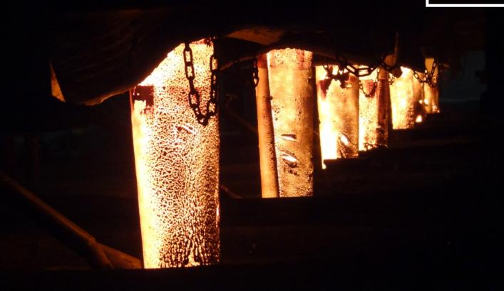
Rarely is reliable uptime so critical, as during continuous casting at a steelworks. To ensure reliable 24/7 operation of continuous casting, system integrator Ingeteam chose VACON® NXP drives to regulate the electromagnetic stirring (EMS) process at the renowned Třinecké železárny a.s., the largest steelworks in the Czech Republic.
