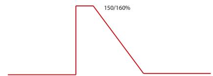
Typical braking profile for horizontal motion (10% duty cycle)
