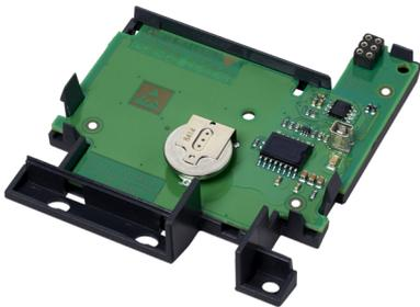
The VLT® Real-time Clock MCB 117 option provides advanced data-logging functionality to the following drives:
