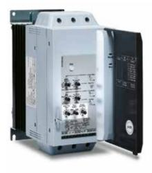
The series offer easy DIN rail mounting for sizes up to 30 kW, 2-wire or 3-wire start/stop control and excellent starting duty (4 x  $I_{e}$  for 6 seconds).
