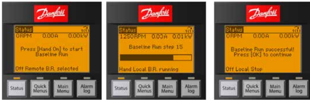
Local operation when enabling the CBM monitoring.
