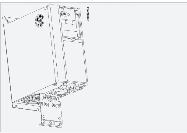
2. Mount the bracket on the decoupling plate.
