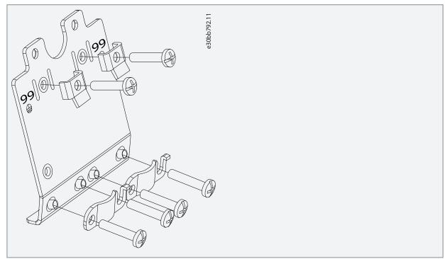
The decoupling plate is now mounted on the drive.
