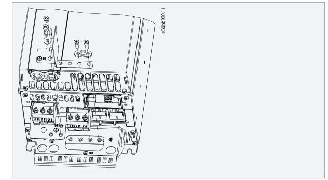
The decoupling plate is now mounted on the drive.
