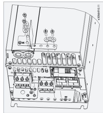
2. Mount the metal plate on the drive and fasten it with the 2 screws provided. Tightening torque: 2 Nm (17.7 in-lb).
