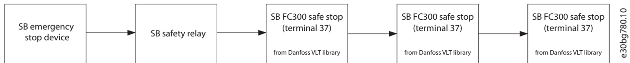
Illustration 5.8 Safety-related Block Diagram
