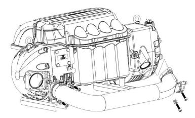
This kit contains the Interstage Pipe as well as the required O-rings and fasteners. Please refer to our Service Manual for details regarding the replacement of the Interstage Pipe.
