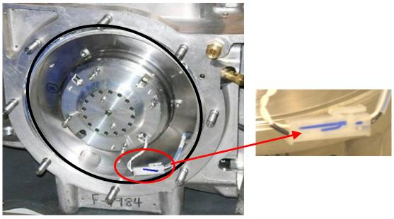
7. Check the seal area (area between red lines) on the End bell for burr, damage or scratches.
