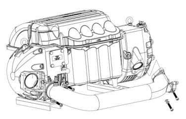
This kit contains the Interstage Pipe as well as the required O-rings and fasteners. Please refer to our Service Manual for details regarding the replacement of the Interstage Pipe.
